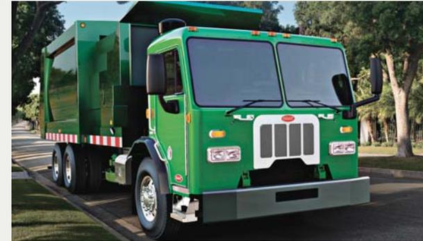
A huck-bolted aluminum cab features lap seam construction and bulkhead style doors on a zinc-coated, steel subframe for maximum durability and corrosion resistance. Use of LED marker lights, instead of incandescents, extend service intervals.
