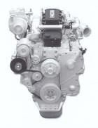
The 8.9-liter PACCAR PX-9 engine has one of the highest power-to-weight ratios in its class, with heavy-duty features like replaceable wet liners, roller cam followers, bypass oil filtration and targeted piston-cooling.
